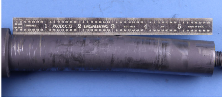
Figure 12. Aft hinge fitting after disassembly showing the bent shaft.
