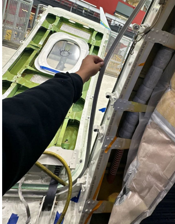
Figure 15. Photo showing the MED plug opened to work on damaged rivets. (Source: Spirit AeroSystems.)
